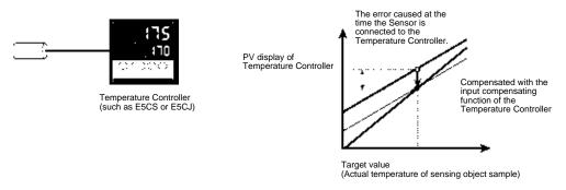
Gain and Offset Compensation with Two-point Compensating Function
